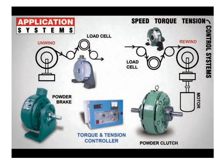
Schematic: Powder Brakes & Clutched are used as Unwind & Rewind Torque control, with Load Cells Dancer & Tension Control, to maintain CONSTANT TENSION.
